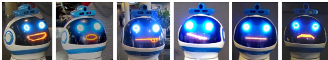
Fig. 13 Different output expressions for robotic emotional interaction
