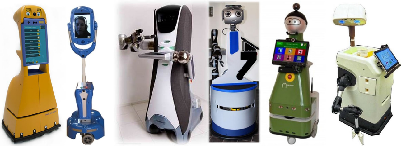
Fig. 1 Robotic platforms developed in the CompanionAble, GiraffPlus, Accompany, Robot-Era, Mobiserv and Hobbit projects (from left to right)
