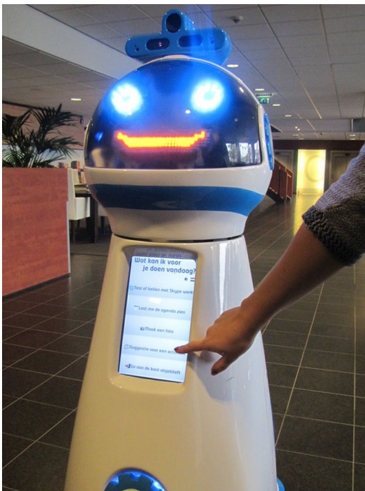
Fig. 8 QT-based user touch interface running on the SocialRobot
