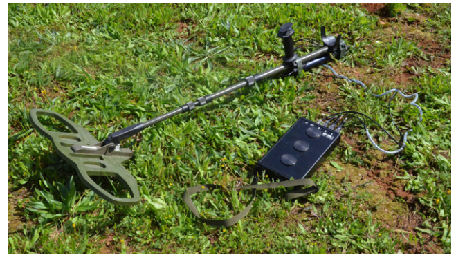
Fig. 18. The original Vallon VMP3, before being modified to fit the arm.
