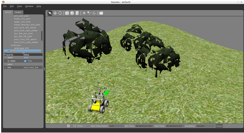
Fig. 14. 3D Gazebo simulation of the FSR Husky in an outdoor environment.
