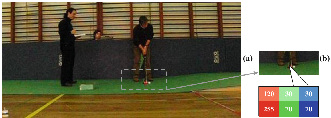
Fig. 3 Example of a registered scene: a full frame, b region of interest with the defined range of RGB values for putter detection
